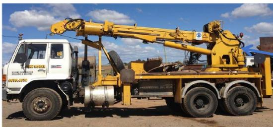
A piling rig for tight access applications was used to bore the piles. This allows piles to be bored from a surface not level with the pile finish level. (i.e. the plant item can site below or above the finish surface level of the piles, which is not achievable utilising a normal piling rig).
